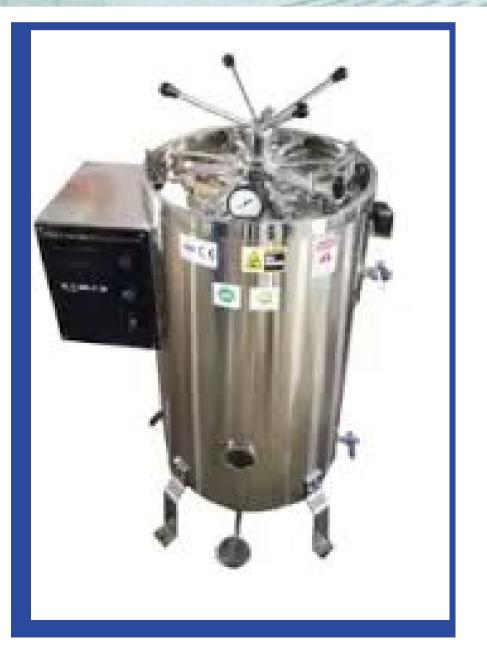
Autoclave, also known as steam sterilizer, is the most effective machine used for the sterilization of lab equipment, water, or media. The machine uses steam under pressure to kill bacteria, viruses, and spores present in/on the equipment or culture media. It is used in scientific labs, healthcare facilities, and industrial operations for the sterilization of a range of tools, vessels, solutions or media, and materials.
