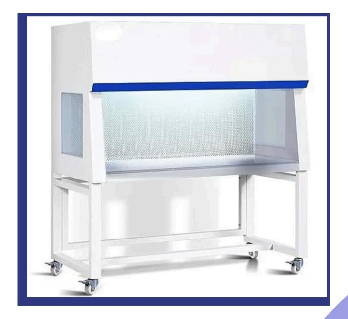
It is the most used type of laminar air flow. In vertical flow cabinet, room air is entered in working area through HEPA filter fitted on top of the cabinet. Thus, air flows downward (vertically) towards work surface and leaves the cabinet sweeping out particles and bacteria.
