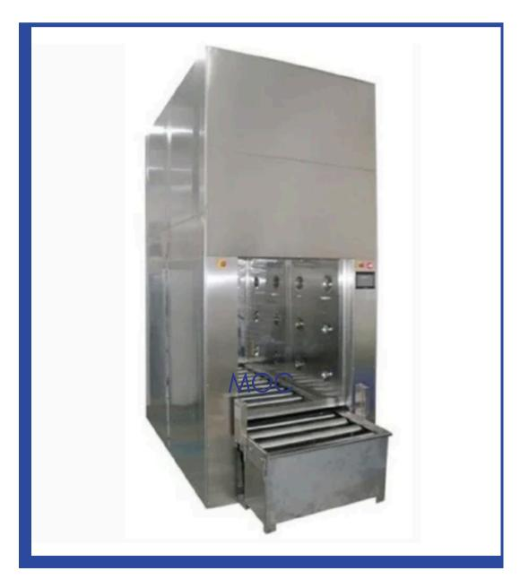
The De-Dusting Tunnel/Booth system is used to remove the loose foreign particles/dust present on the received material, which are brought into the warehouse before they area transferred into the quarantine area. Motorized roller conveyor transfers heavy load material from material loading area to de-dusting chamber and then finally to the material unloading side.
