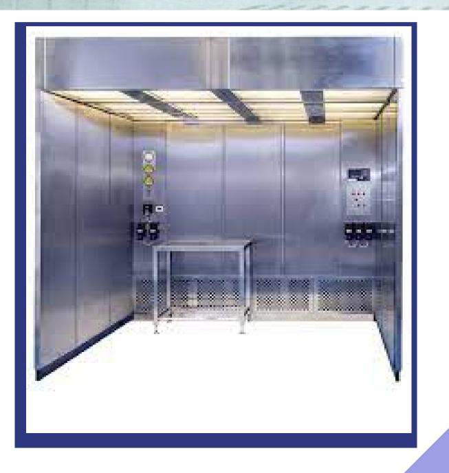
Reverse Laminar is an exclusive clean containment enclosure for bulk powder or liquid weighing, sampling, mixing or dispensing. The self contained, free standing booth provides localized protection of product or personnel when handling non - potent bulk materials.
